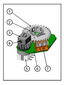
The "customer" terminal must be connected with rigid wires. If the applied voltage is higher than 42V, the user must foresee a fuse in the power supply line.
